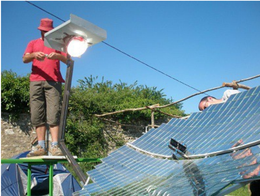
Example of a Scheffler reflector, built for experimentation and training
